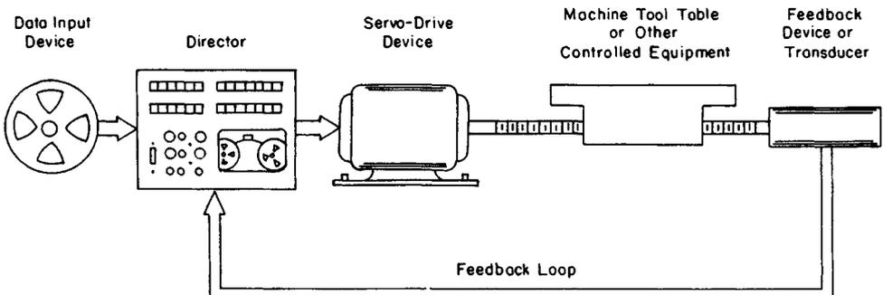
Fig. 37.4 Simplified numerical control system.
