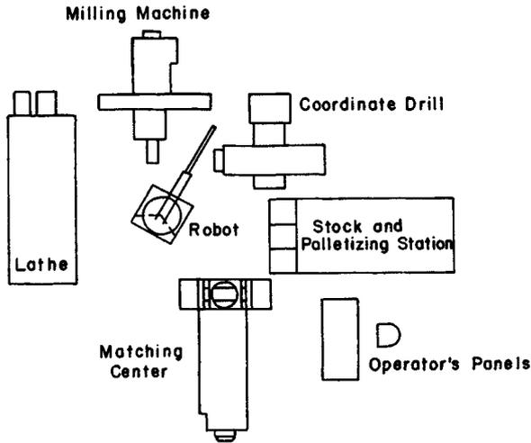
Fig. 37.10 A typical manufacturing cell.
