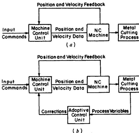
Fig. 37.6 Schematic diagrams for conventional and adaptive NC systems.
