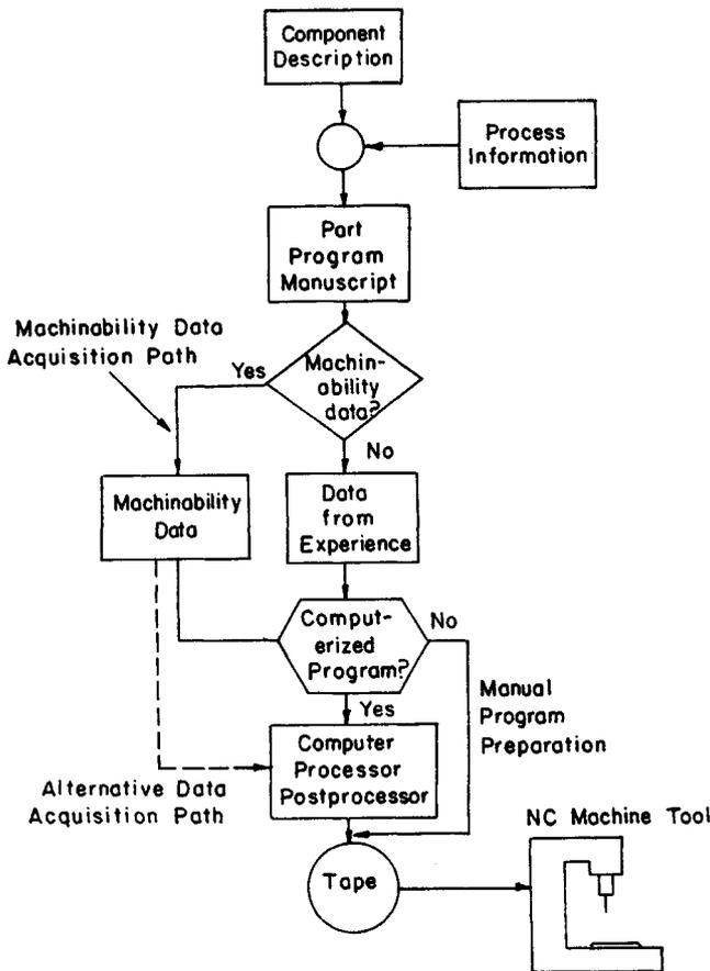
**Fig. 37.7** Acquisition of machinability data in the NC process flow.
