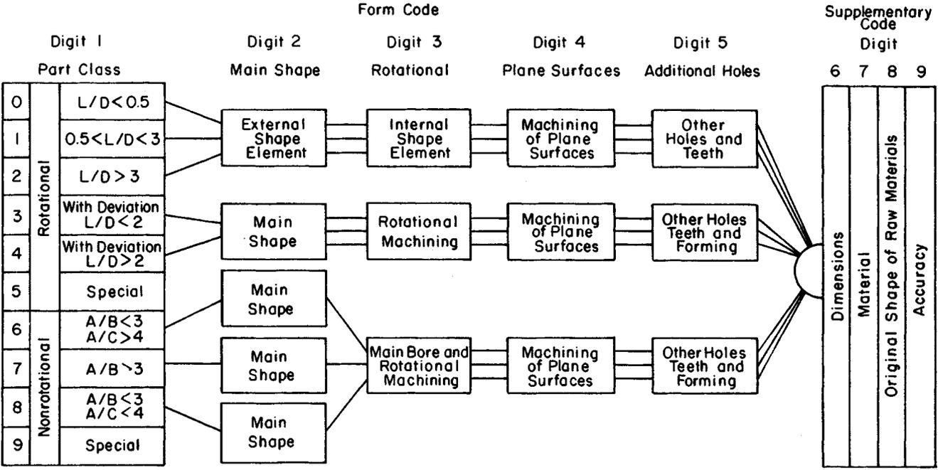
Fig. 37.12 Opitz parts classification and coding system.
