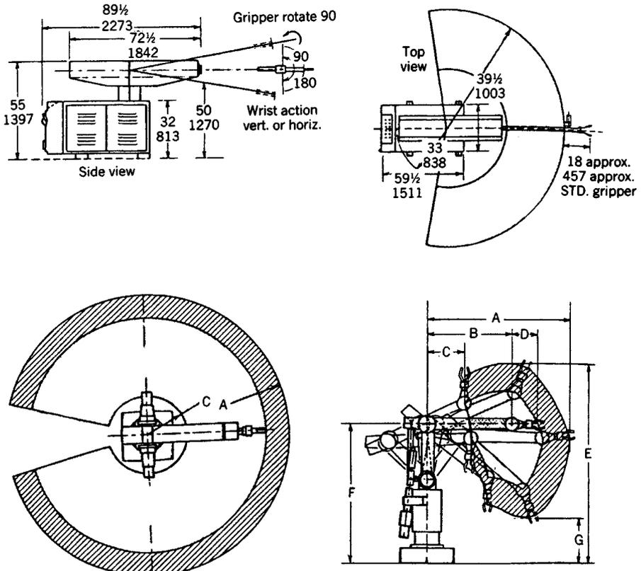
Fig. 37.8 Mechanical configurations of industrial robots.
