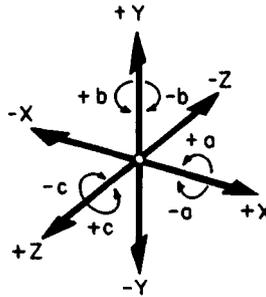
Fig. 37.5 An example of typical axis nomenclature for machine tools.
