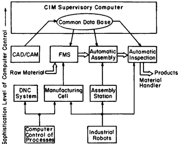
Fig. 37.9 Hierarchical computer control in manufacturing.
