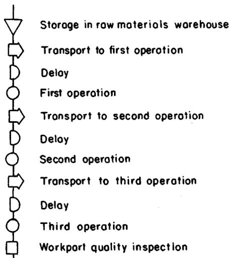
Fig. 37.2 Flow process chart for a sample workpart.
