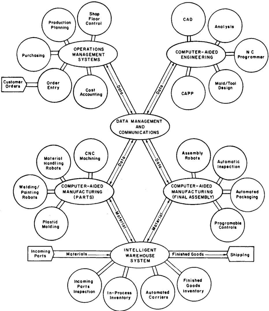
Fig. 37.1 Computer-integrated manufacturing system.
