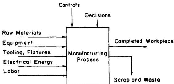
Fig. 37.3 General input-output model of the manufacturing process.
